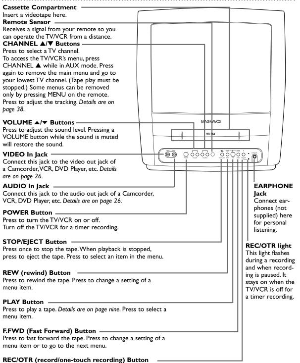
Press once to start a recording. Details are on page 10. Press repeatedly to start a One-Touch Recording (an immediate timed recording, 30 minutes to eight hours long) of the current TV channel. Details are on page 27.
